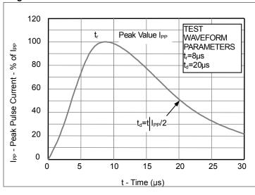
Fig2. ESD Pulse Waveform (according to IEC 61000-4-2)
